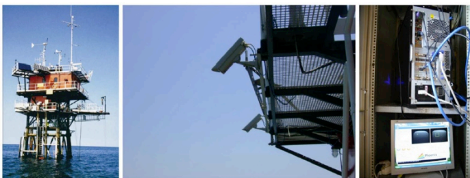
Fig. 1 - Left: CNR-ISMAR oceanographic platform Acqua Alta off the Venice coast in Italy. Center: deployed WASS . Right: WASS data acquisition workstation.
